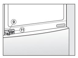
■ Fit hinge pin ⑨ into middle hinge plate ① in the lower door.
